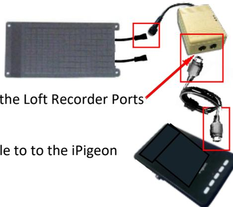
Using either end of the Mini-DIN cable connect to either of the Loft Recorder Ports
