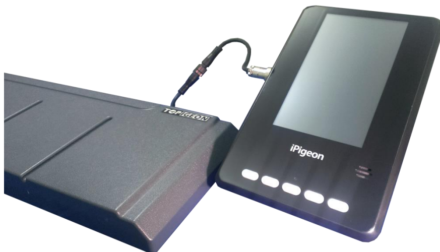
iPigeon and loft antenna connection
