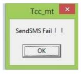
If the phone testing fails, you should restart the GSM module power. Then, restart the SMS program and run the phone testing, until you success.
