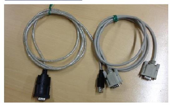
Most of PC now does not provide RS232 port. Then you need a USB to RS232 convert cable. When you installed the USB driver, you will see the Ports setting in the device Manager panel listed of "Profilic USB-to-Serial Comm Port(com X)" •
